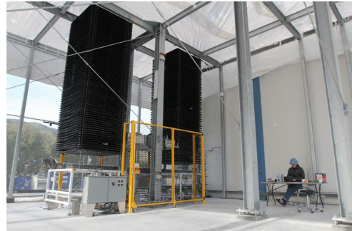
Equipment holding trays of limestone is part of a carbon-removal process developed by Heirloom Carbon. PHOTO: NATHAN FRANDINO/REUTERS
