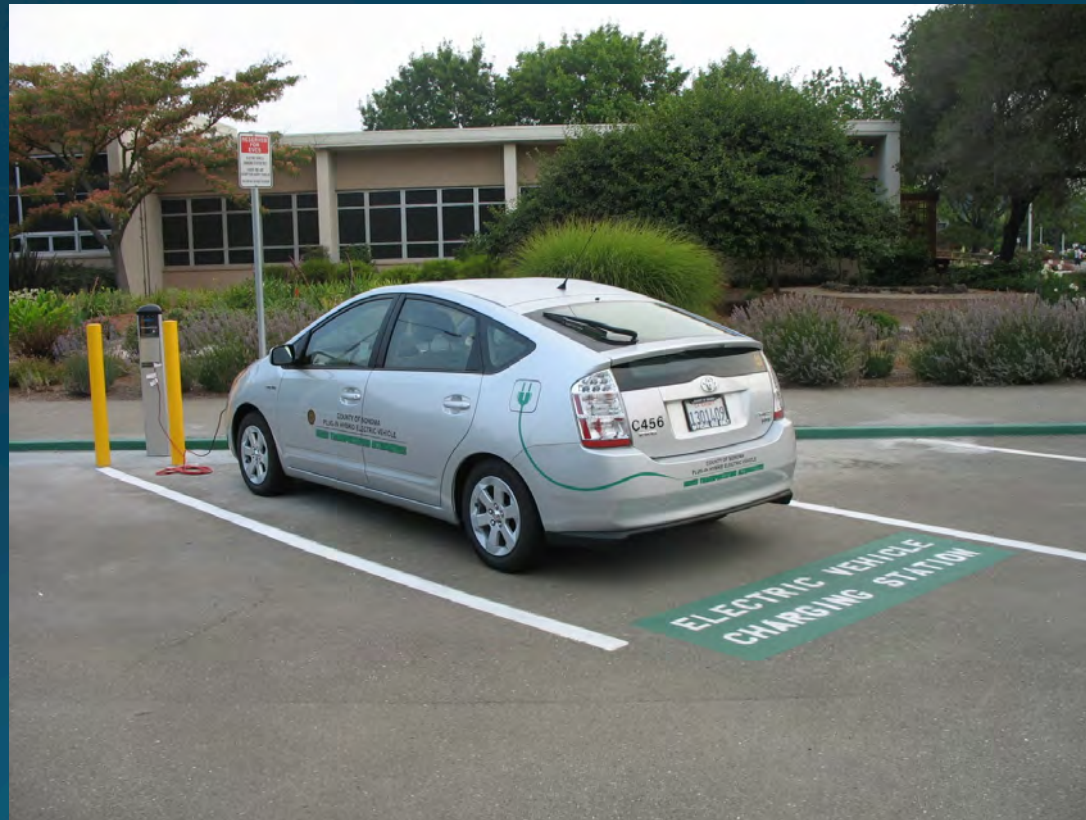
2009 Toyota Prius Converted to a Plug-In Hybrid EV
